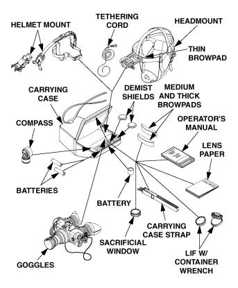
Figure 1-1. Night Vision Goggles (NVG), AN/PVS-7B and AN/PVS-7D (Sheet 2 of 3).
